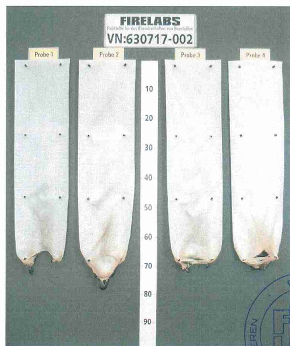
fig. 4 View of test specimen after the test (sample no. 4: rear side)
